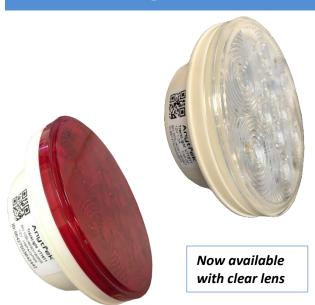
The lamps meet all FMVSS P2 photometric requirements for visibility and safety. Lenses and housings are made of tough ABS material and are ultrasonically welded. The lamps employ a solid state, surface-mount device design that protects the electronics against moisture, shock, and vibration.
